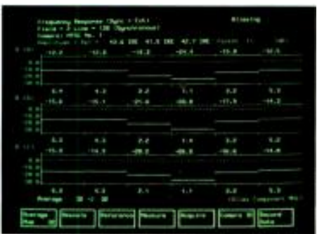
Figure 7. Frequency response tests of red, green and blue channels also show aliasing.
