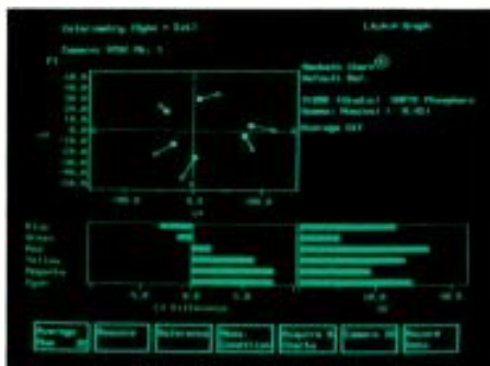
Figure 2. The deviation in output from a single patch of the test chart is shown on a CIE 3-D color space triangle.
